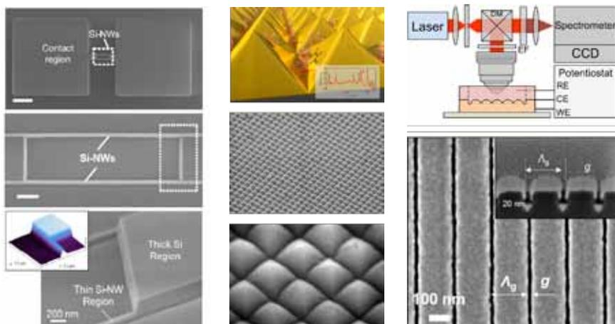
Silicon nanowires (left), gold nanopillars (middle) and nano-interdigitated electrodes for electrochemical SERS (right)
