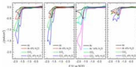
(Right): Rh complexes investigated in this study. (left): cyclic voltammograms of 1 mM of compounds 1, 2, 3, and 1' (left to right) in MeCN with 0.1 M Bu<sub>4</sub>NPF<sub>6</sub> under argon or CO<sub>2</sub> and with or without water
