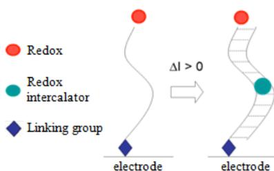
Figure 1: Scheme of a long range electron transfer RNA biosensor with redox intercalator
