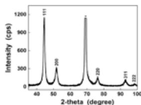
Fig.1. SEM and XRD characterization of NiNP
