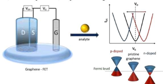
Figure 1: Needle type graphene-FET architecture used for the detection of different analytes
